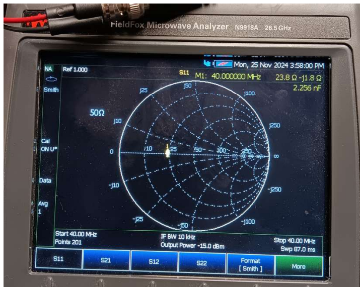
Figure 8: This was our matching network with an unmatched arbitrary load at 40 MHz.
