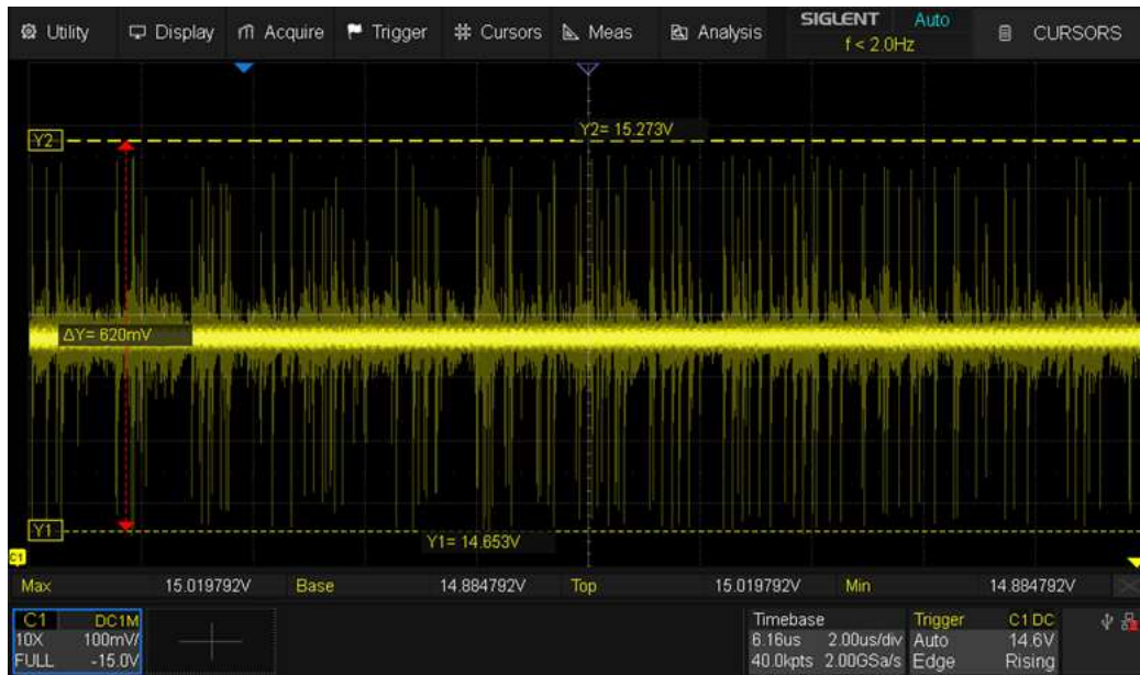
Figure 25: Noise in circuit due to laptop being connected on the same power outlet.
