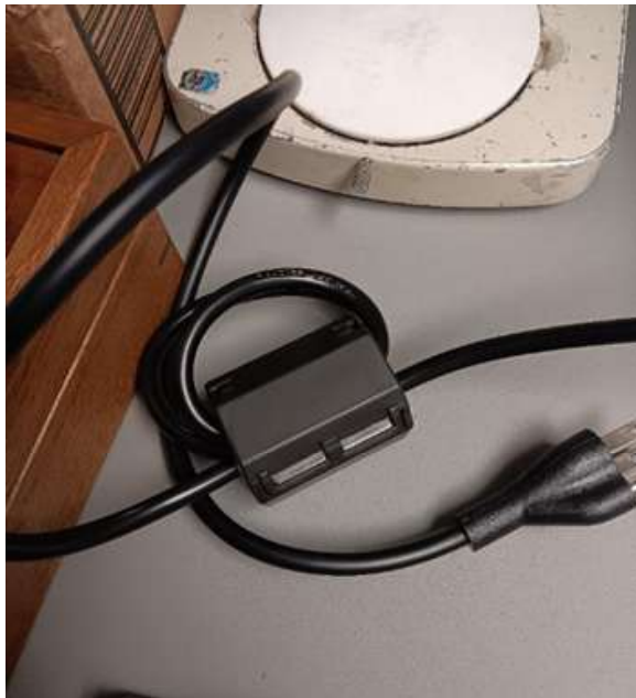
Figure 26: Added this ferrite toroid on the power cord running to the oscilloscope, wrapping the cord three times inside it helped reduce the noise considerably.
