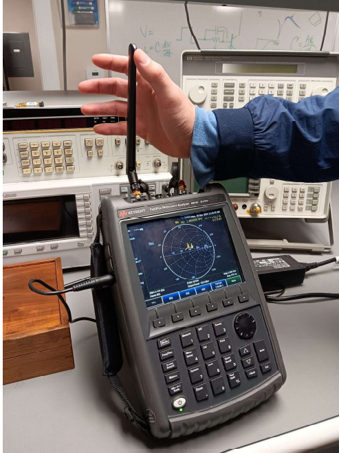
Figure 3: Testing our antenna. Viewing the S11 parameter change on Keysight FieldFox as hand movements were made.
