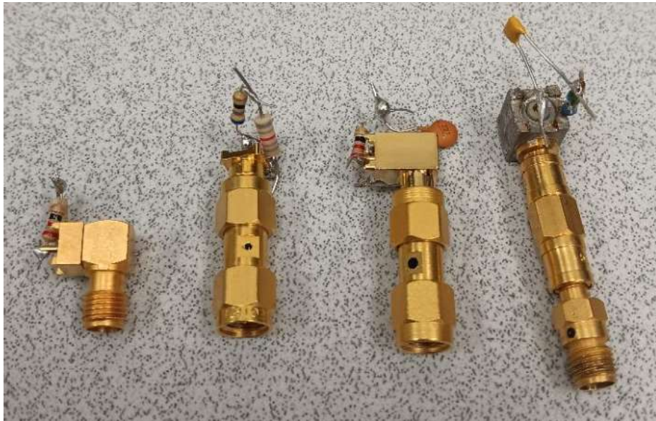
Figure 6: Arbitrary loads created to practice impedance matching and develop our algorithm.
