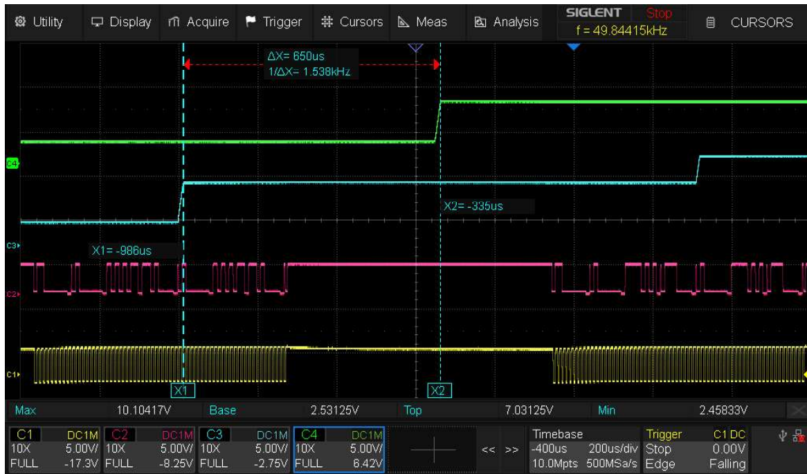
Figure 15: Same results as in figure 14. The cursors here are used to measure the delay between both outputs OP1 and OP2.
