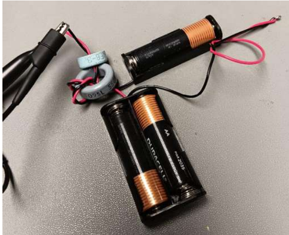
Figure 27: Using AA batteries with ferrite toroids on the power leads to power the Curiosity Nano and adding two 470uF capacitors and one 100uF capacitor at boost module output rail we achieved a noise floor of \sim 5\text{mV} . We could not get it better than this.
