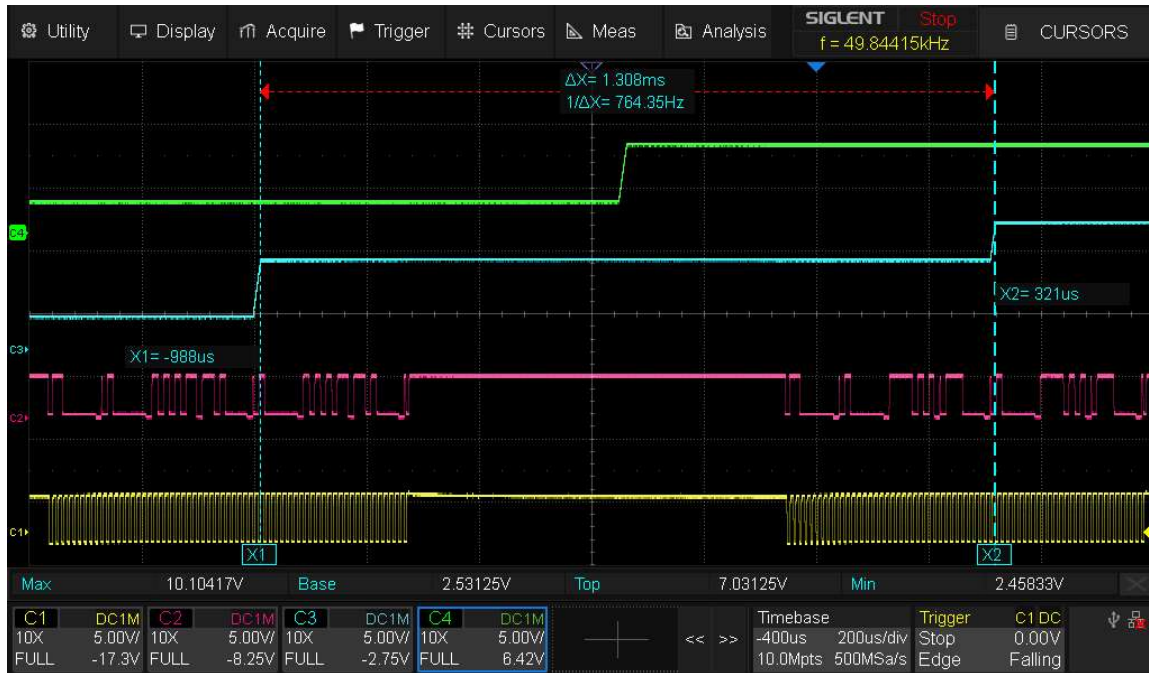
Figure 14: Oscilloscope results of testing the DACs. The yellow waveform is the SCL (clock) line of DAC1, the pink waveform is the SDA (data) line of DAC1, the blue waveform is the output OP1, the green waveform is the output OP2. Note: the points where the data line is pulled to zero are the ACKs (acknowledgments sent from the client to the host).
